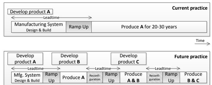
Fig. 1. Reducing of leadtimes by using RMSs [2]
