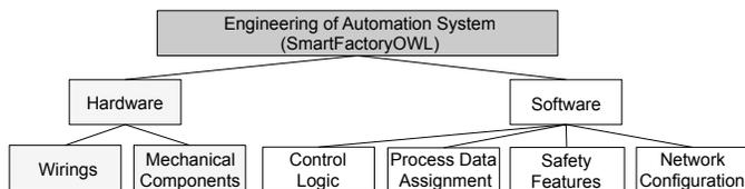
Fig. 4. Identified engineering categories needed for the setup of the SmartFactoryOWL
